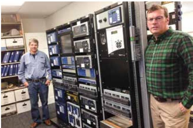
Kevin Coyne, integration engineer Casco Systems and Kevin Mahoney, founder and President of Casco Systems, with the IEC-61850 Simulation System used for Research and Development. This lab configuration was used to prototype and validate all of the integration and protection settings for the project.
